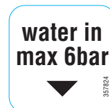
To avoid damage, do not exceed a water pressure of 6 bar.
