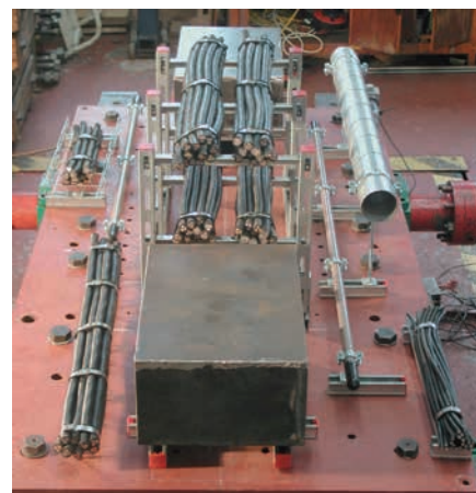
Test configuration: Two base plates were populated with MQ channel fastened with X-BT studs. The base plates were rigidly attached to the 2-tonne shock loading machine.
