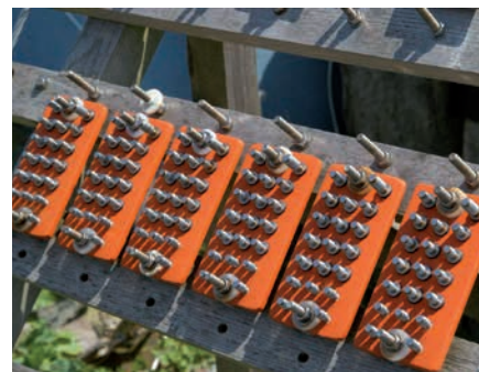
Marine atmosphere test rig with X-BT test specimens installed.
