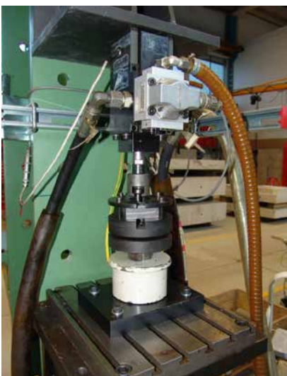
Servo-hydraulic test setup for tension fatigue tests
