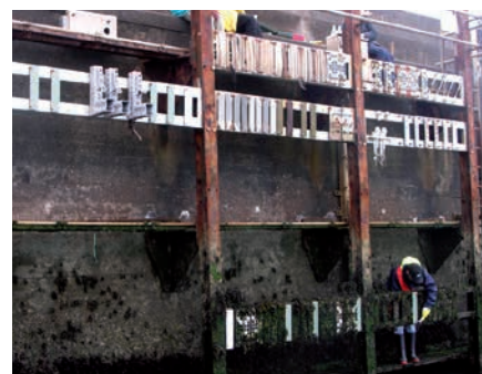
Sea water test rig with test specimens installed (X-BT with and without X-FCM grating discs).
