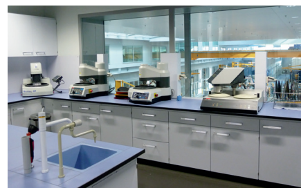
Fig. 23: Metallographic laboratory equipment (grinding and polishing).
