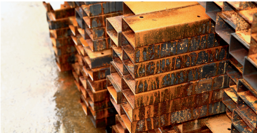
Fig. 4: Corrosion of steel components.
